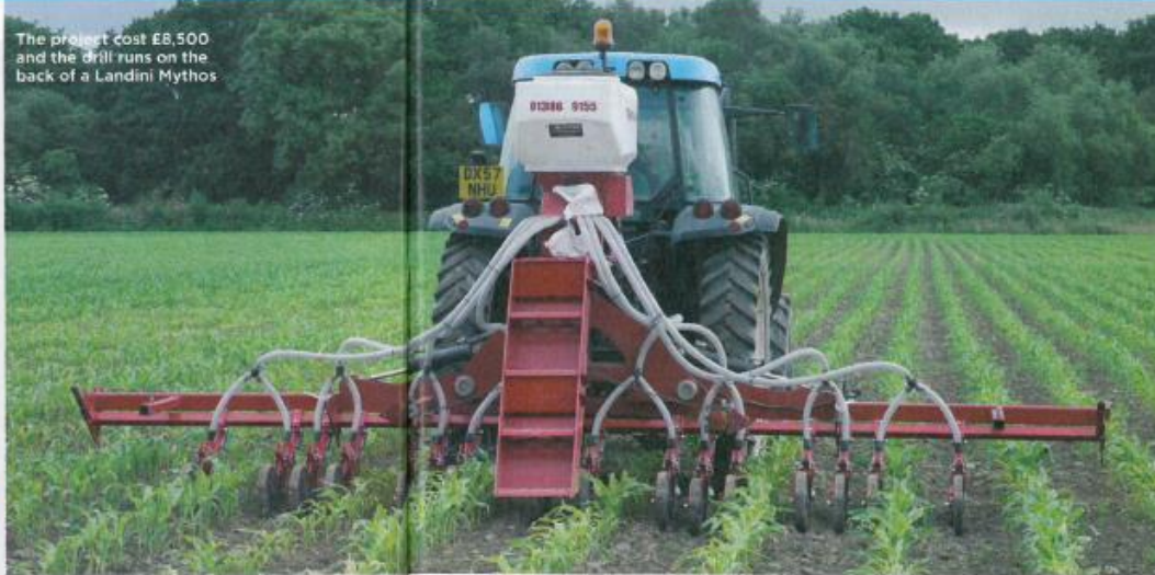
A combination of disc coupler and press wheel get the crop in the soil
